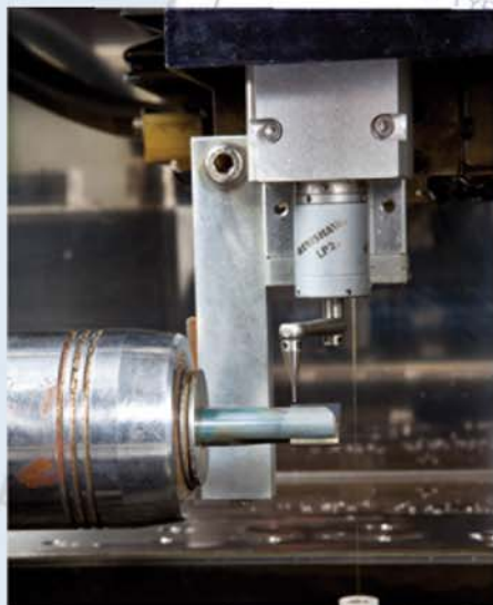
Dedicated EDM for cutting special tools intricate contours
